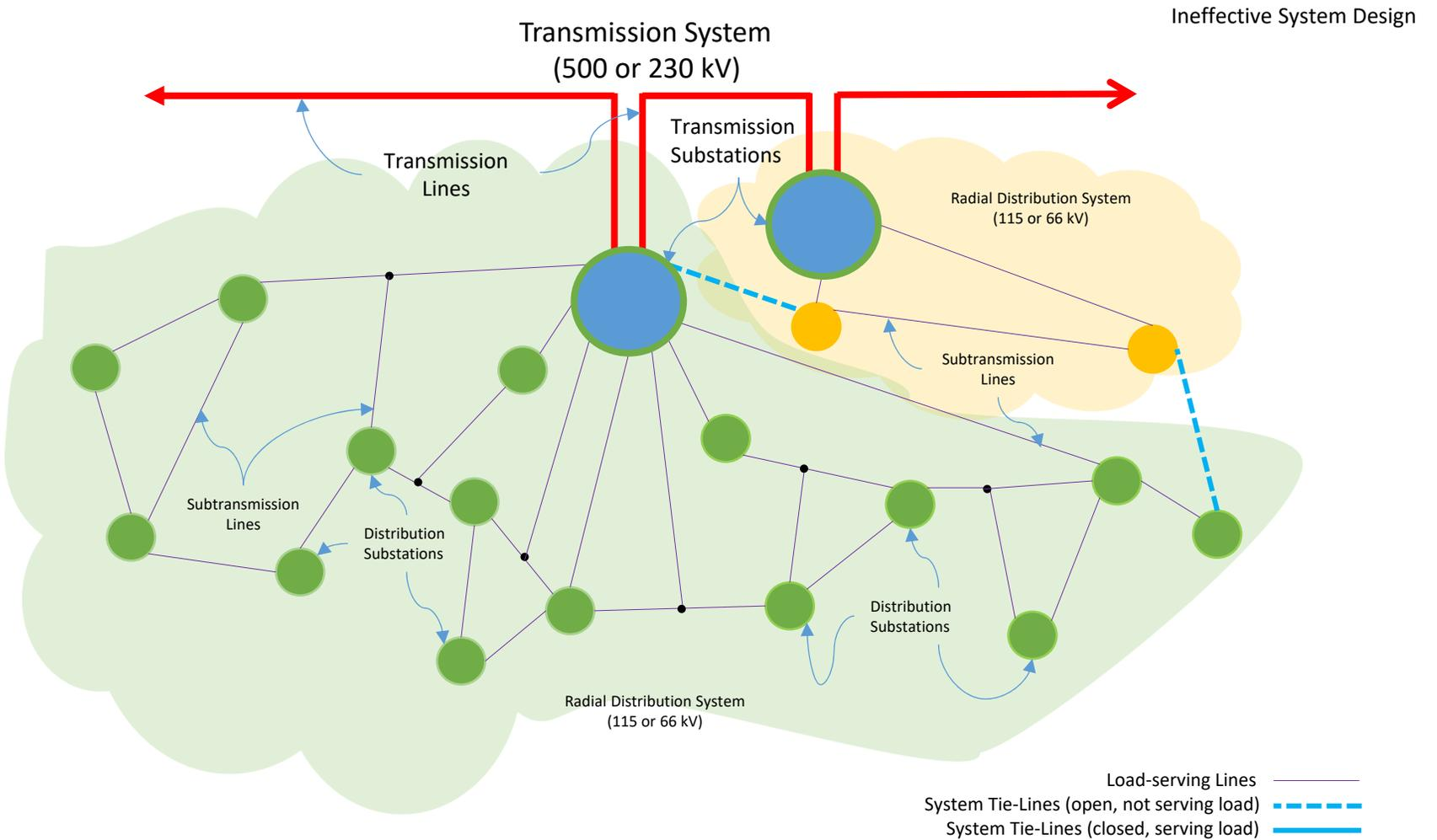
(2) Radial Distribution Systems with *ineffective* system tie-lines *not* located “downstream” at the intersection of the two systems thus not allowing for bi-directional transfer of substations without interfering with the reliable and safe operation of the remaining network following the transfer.
