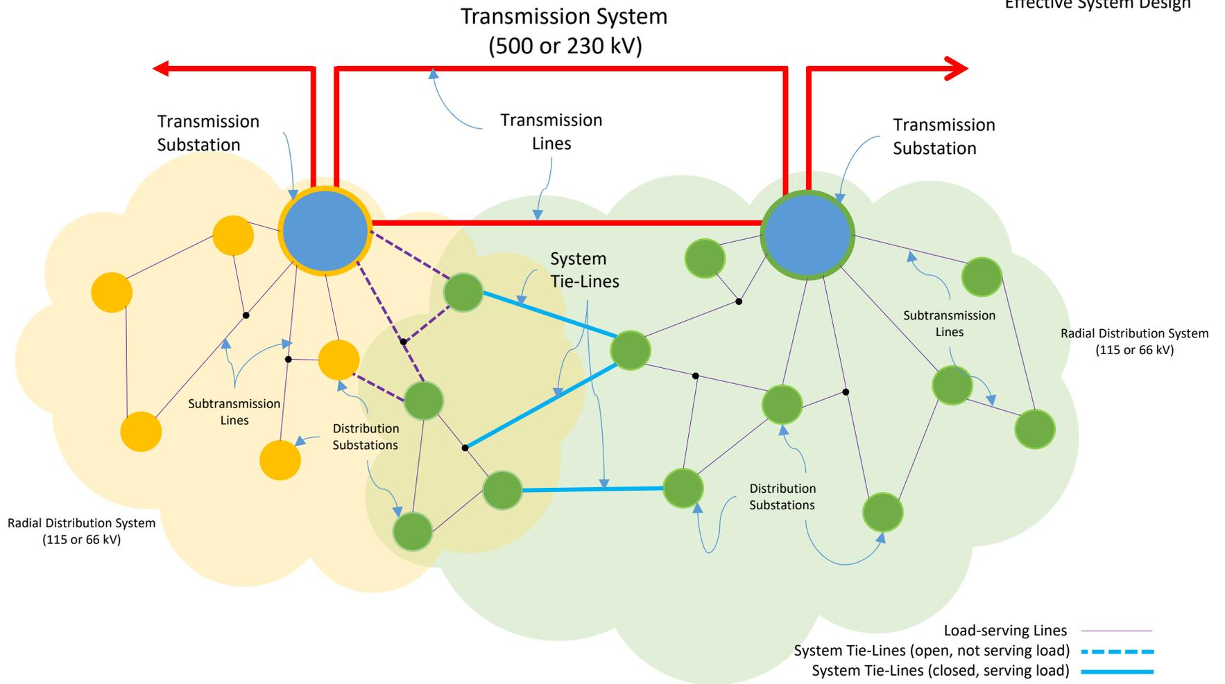
(2) Radial Distribution Systems with *effective* system tie-lines. Following an incident on the system to the left, the system on the right is able to effectively transfer significant load from the system on the left to provide relief and improving reliability and resiliency.
