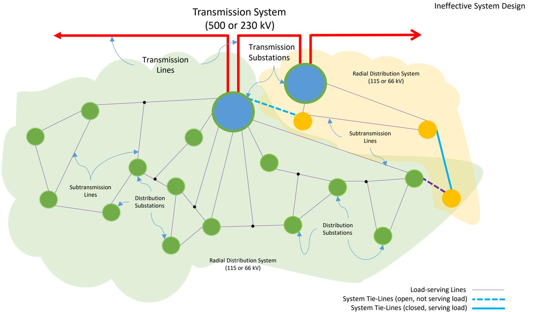
(2) Radial Distribution Systems with *ineffective* system tie-lines *not* located “downstream” at the intersection of the two systems thus limiting bi-directional transfer of substations without interfering with the reliable and safe operation of the remaining network following a transfer.
