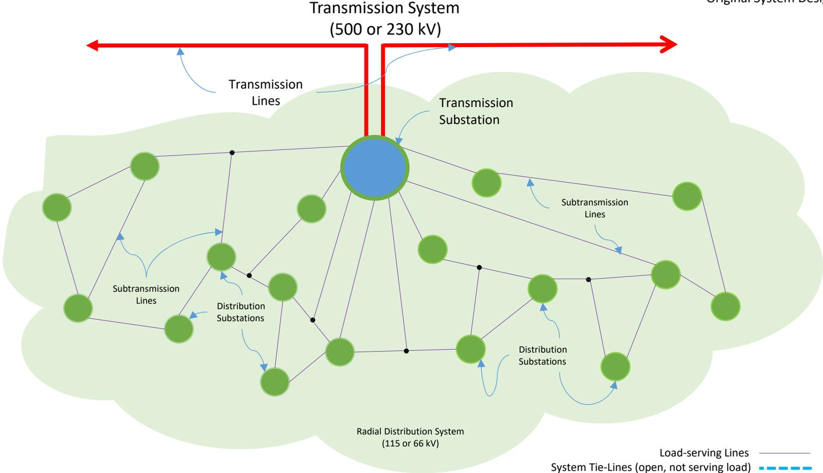
Radial Distribution System with no system tie-lines
